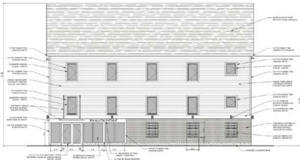
Figure 10: Proposed front elevation for office building
